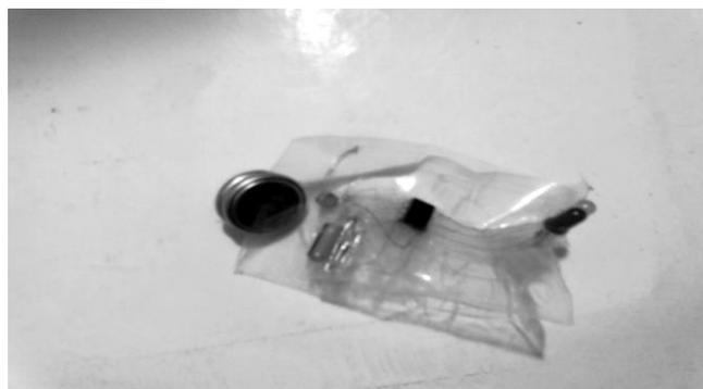
Fig.4. Our flexible PCB prototype in crumbled condition
