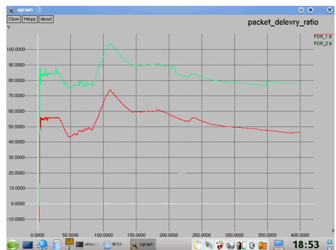
Figure 4 shows that packet delivery ratio of simulated node in given scenario of AODV Protocol and AODV-OSPF routing protocol.
