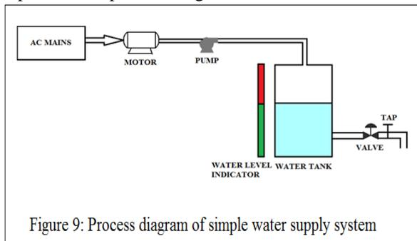
Figure 9: Process diagram of simple water supply system
