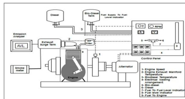
**Figure 1. Schematic diagram of experimental test rig setup**
