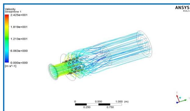
**Figure 4.5:** Velocity Streamline For Silencer With 24 Holes Of Rectangular Extrusions Of 30\*40 Mm Dimension And 20mm Height.
