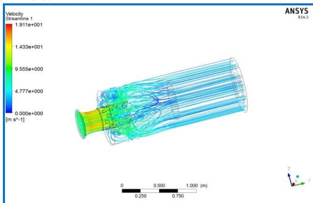
**Figure 4.3:** Velocity Streamline for the Silencer with 24 Number of Rectangular Holes of 30\*40mm Dimension.
