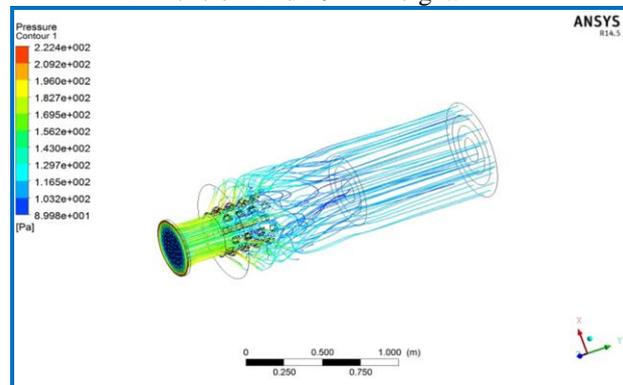
**Figure 4.6:** Total Pressure At The Inlet And Outlet For Silencer With 24 Holes Of Rectangular Extrusions Of 30\*40 Mm Dimension And 20mm Height.
