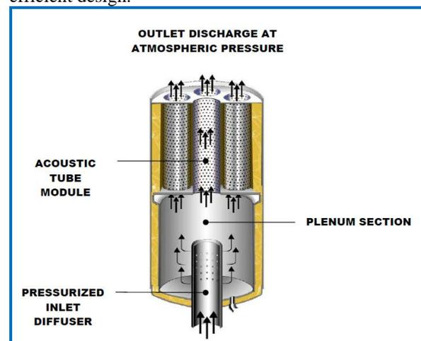
Fig -1: Absorptive type of silencer
