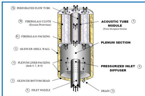
Fig -2: Typical Absorptive silencer with parts
