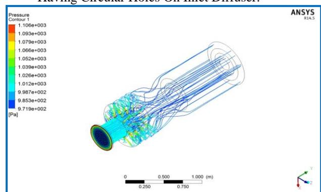
Figure 4.2: Total Pressure Distribution At The Inlet And Outlet For The Model Having Circular Holes On Inlet Diffuser.
