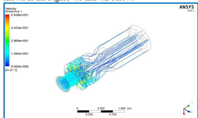
Figure 4.1: Velocity Streamlines For The Model Having Circular Holes On Inlet Diffuser.
