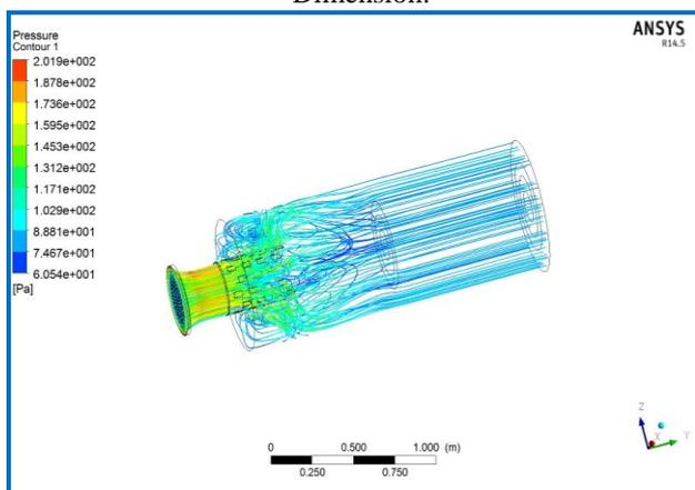
**Figure 4.4:** Total Pressure Distribution At The Inlet And Outlet For The Silencer With 24 Number Of Rectangular Holes Of 30\*40mm Dimension.
