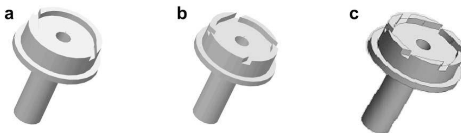
Fig. 6 – Nozzles used in experiments: (a) 2 nozzle, (b) 4 nozzle, and (c) 6 nozzle
