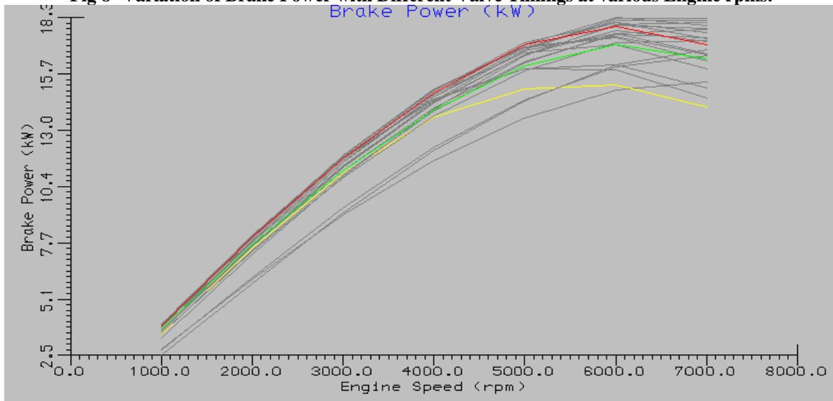
The above Graph indicates that Brake Power, BSFC and BMEP are indeed dependent on the Volumetric Efficiency as the graph with higher BP indeed is the one with higher Volumetric Efficiency (Red)
