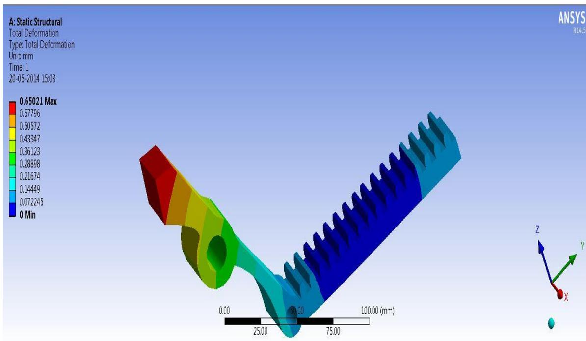
**Fig.4-Ansys Structural Deformation Analysis of Rack with Lever Arm**
