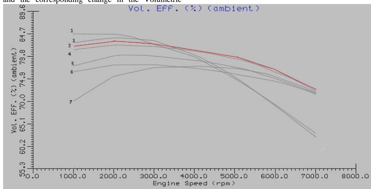
Fig 3 – Volumetric Efficiency curves for optimum Inlet valve opening and closing angles.
