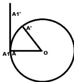
The above circle represents the pitch circle of the pinion gear and the tangential line drawn to it at the left is the rack respectively. Let A be a point at the circumference of the pinion meshing with the corresponding point A1 on the rack. Thus as the rack moves up linearly due to the servo motor rotation for the valve actuation, the point A1 reaches point A1'
