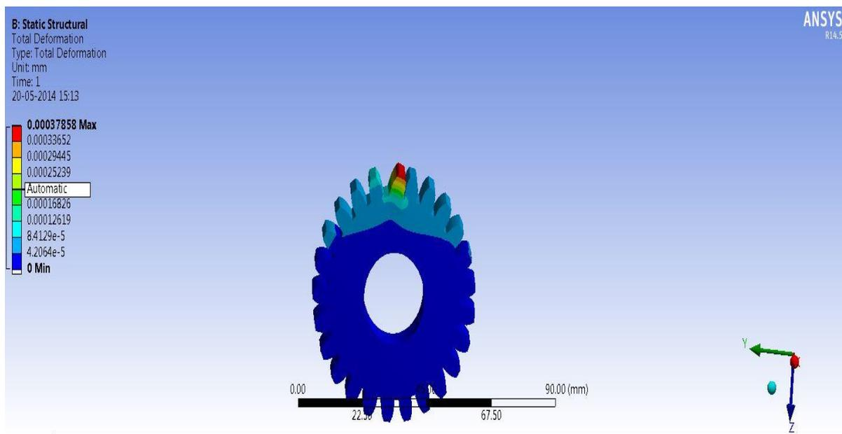
**Fig.5- Ansys Structural Deformation Analysis of Pinion Gear**
