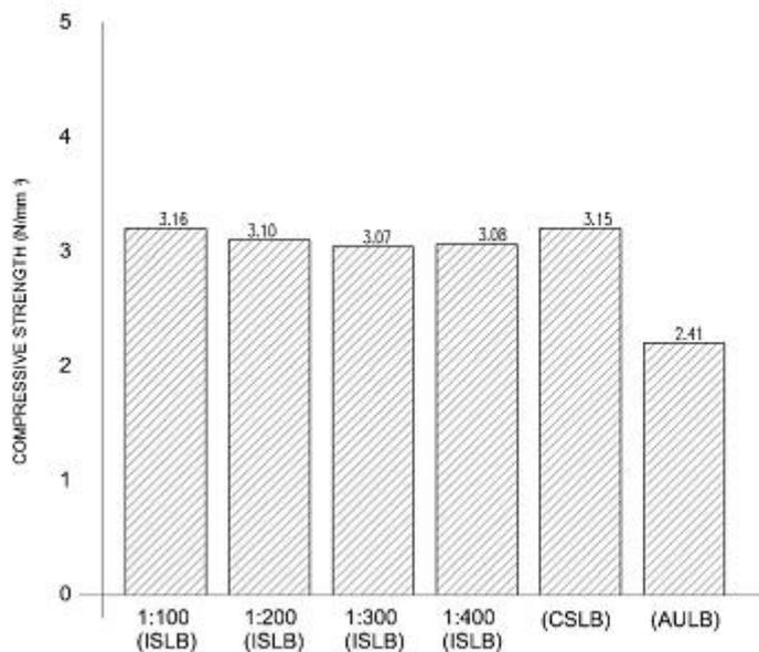
Figure 1.0 Compressive Strength Test Result for Brick Specimen.
