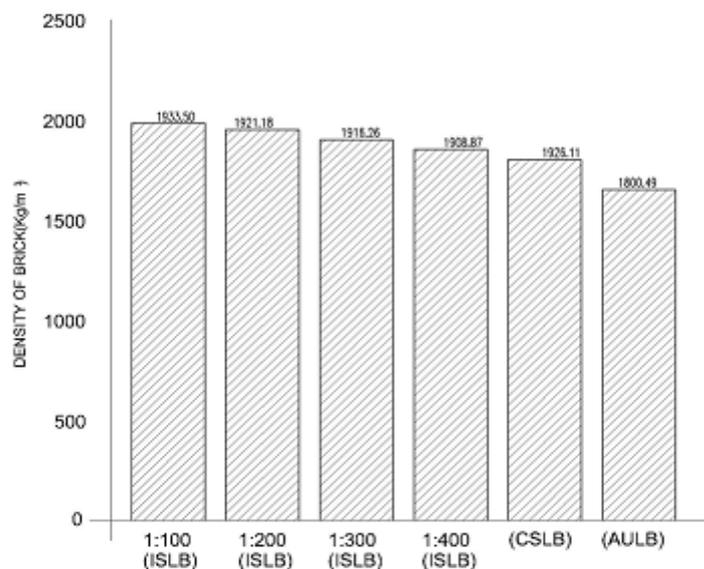
Figure 2.0 Density Test Results for Brick Specimen.
