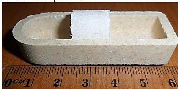
Fig. 1: Composite pellet (of Al<sub>2</sub>O<sub>3</sub> + PS) utilized for thermal decomposition of PS at 1550 °C
