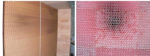
Figure 3. Two methods for the honeycomb: cooling pad (left) and straws (right).
