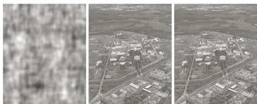
1) Comparison result of a) Full inverse b) Radially inverse c) Wiener filter
