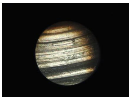
Fig.4. Wear Pattern on the Ball Surface
