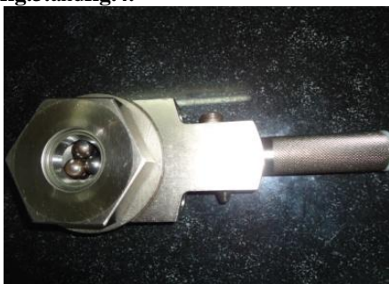
Fig.3. Experimental Balls in the Ball Pot
