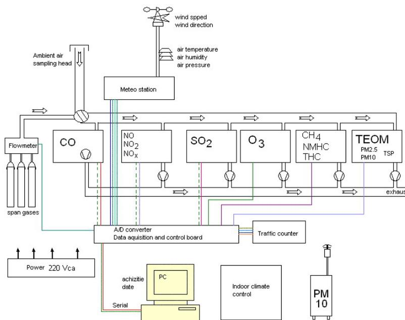
Figure 2. The Schematics of the AQM Mobile Station.
