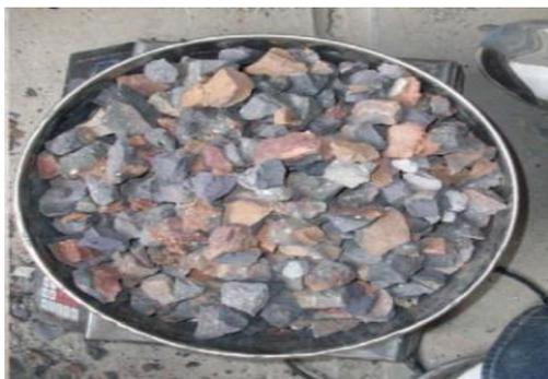
**Figure 1:** Over Burnt Brick Ballast Aggregates
