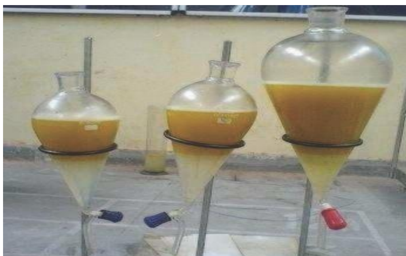
Figure 4: Washing process of biodiesel.
