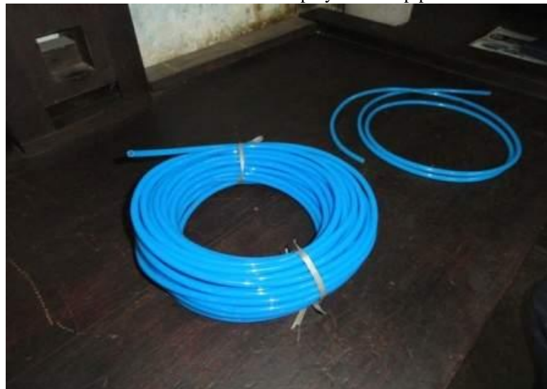
Fig. Polyurethane pipe as void former 6mm outer diameter
