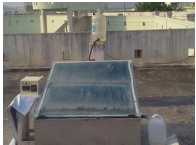
Fig. 4: Complete Experimental Setup of Solar Still
