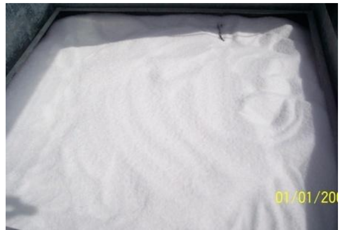
Fig. 3: PCM in Heat reservoir
