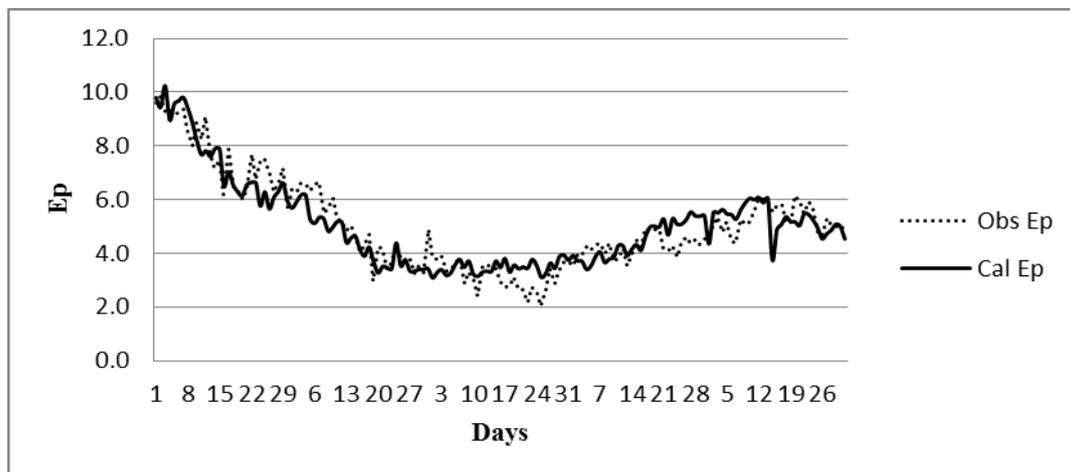
Fig. 8 Performance of fitted Jensen equation in Calibration
