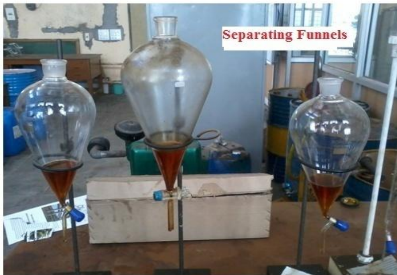
Figure 6: Glycerol separation process
