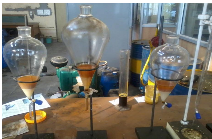
Figure 7: Water washing process of bio-diesel
