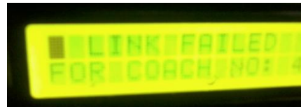
When the connection of compartments failed.
