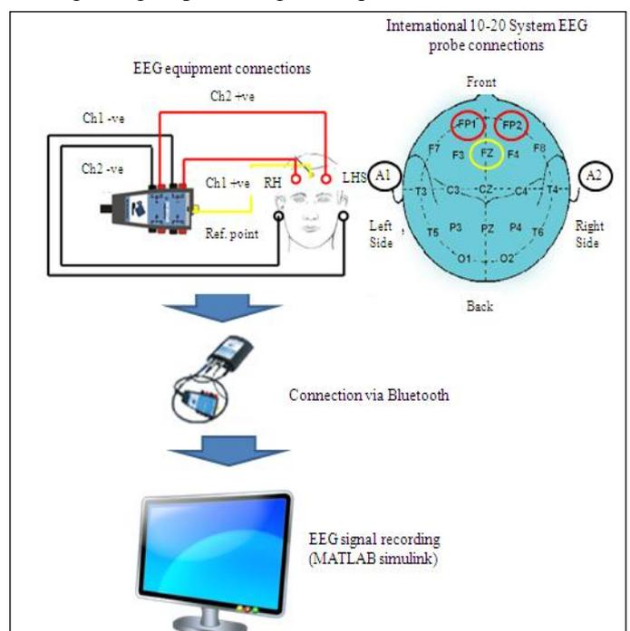
Figure 2. Experimental setup
