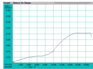
Fig 6: Stress–Strain curve for 6 % Al_2O_3 Tensile strength: 102 N/mm 2 % Elongation: 8.143%
