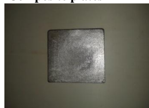
Fig 3.2 Aluminium+6% Al 2 O 3
