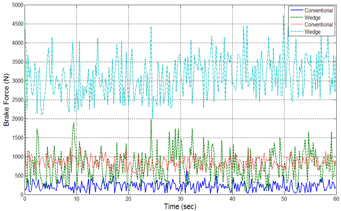
Fig.16 Variation of brake force with time for conventional and wedge disc brake at different applied force
