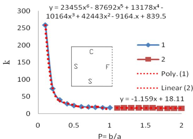
Figure 3: Graph of CSSF Panel  $P = a/b$  (note:  $y = k$  and  $x =$  aspect ratio,  $p$ )
