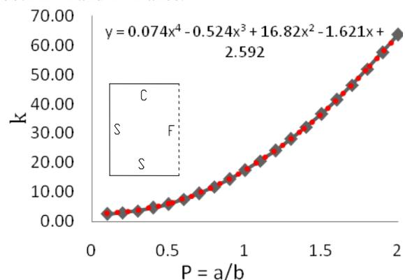
Figure 1: Graph of CSSF Panel P = a/b (note: y = k and x = aspect ratio, P)
