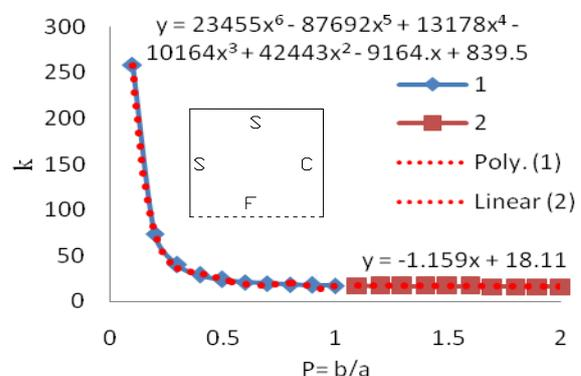
Figure 6: Graph of SSFC Panel  $P = b/a$  (note:  $y = k$  and  $x =$  aspect ratio,  $p$ )
