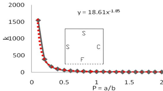
Figure 7: Graph of SSFC Panel  $P = a/b$  (note:  $y = k$  and  $x =$  aspect ratio,  $p$ )
