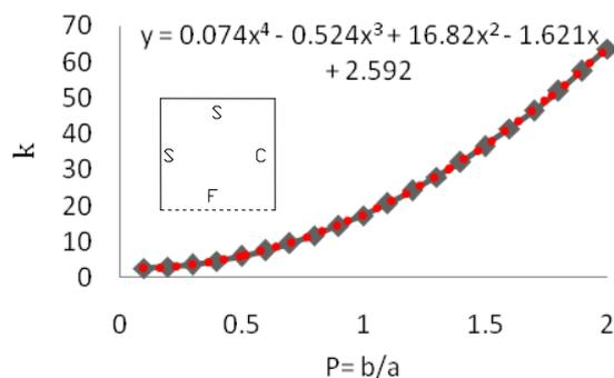
Figure 8: Graph of SSFC Panel  $P = b/a$  (note:  $y = k$  and  $x =$  aspect ratio,  $p$ )
