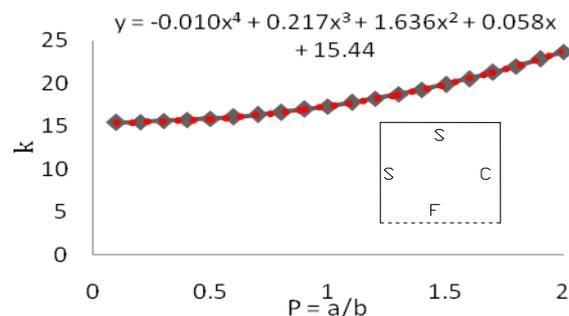
Figure 5: Graph of SSFC Panel  $P = a/b$  (note:  $y = k$  and  $x =$  aspect ratio,  $p$ )
