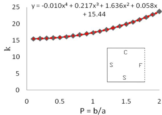
Figure 4: Graph of CSSF Panel  $P = b/a$  (note:  $y = k$  and  $x =$  aspect ratio,  $p$ )
