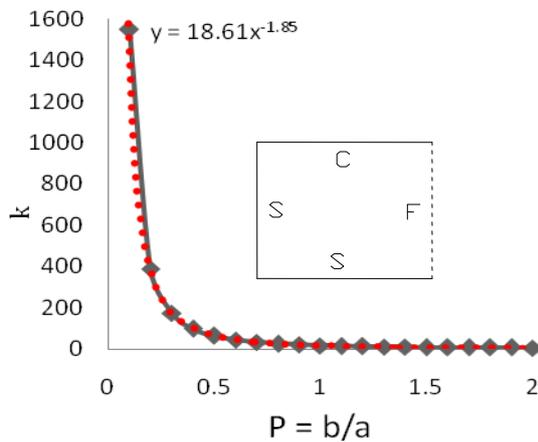
Figure 2: Graph of CSSF Panel  $P = b/a$  (note:  $y = k$  and  $x =$  aspect ratio,  $p$ )
