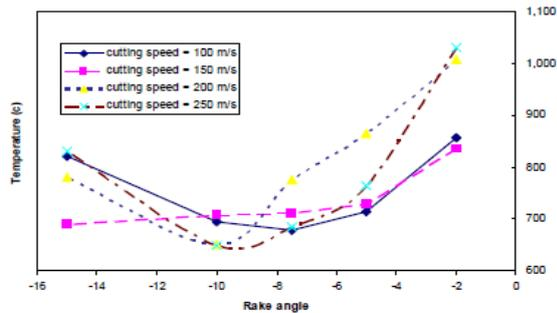
Figure 5: (a) The temperature along tool surface for different rake angle at the cutting speed of 200 m/min and (b) The effect of tool rake angle and cutting speed on predicted cutting temperature.
