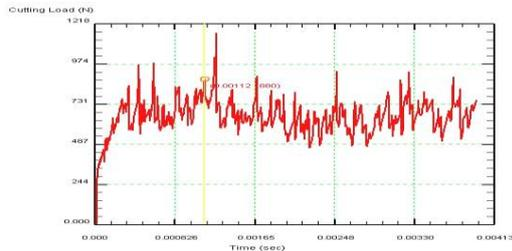
Figure 4: a) The predicted cutting force compare with the experimental cutting forces by Yen, Y-C, Jain, A, Altan, T (2004) of 850 N at the same conditions.
