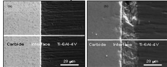
Fig. 3. SEM micrographs of the diffusion couple (a) before and (b) after heating in air atmosphere for 90 min at 800 °C.
