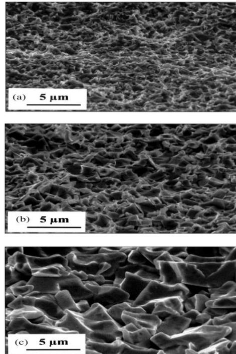
Fig. 1. Surface morphology of 1 mm- (panel a), 3 mm- (panel b) and 6 mm-grained (panel c) WC-Co substrates submitted to two-step chemical etching with Murakami's reagent and H<sub>2</sub>O<sub>2</sub>qH<sub>2</sub>SO<sub>4</sub>.
