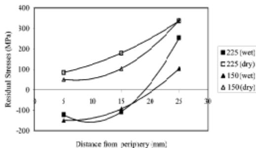
Fig. 6. Effect of coolant on the residual stresses for CBN (C1 type) cutting tool at two different cutting speeds (150 and 225 m/min; 0.15 mm/rev; 0.5 mm) at 5, 15 and 25 mm from the periphery.
