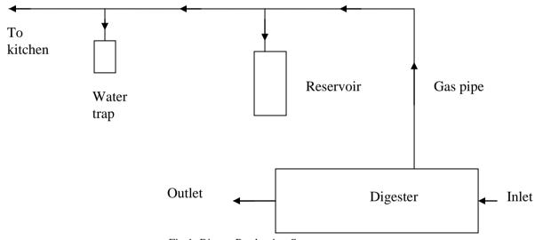
Fig.1: Biogas Production System
