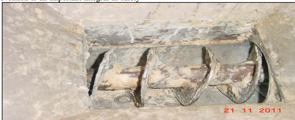
Fig 2: The extruder shaft welded screw joint
