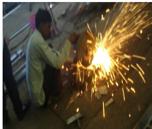
Fig 2: Cutting of sample from strip
