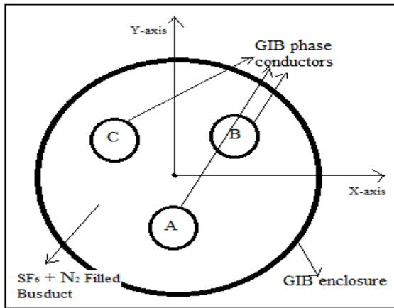
Fig.1. Typical three phase common enclosure Gas Insulated Busduct.
