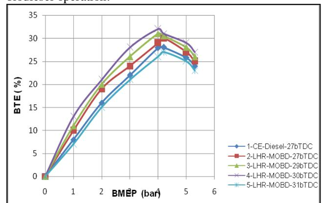
**Fig. 4 Variation of BTE with BMEP in LHR engine at different injection timings with biodiesel (MOBD) operation.**
