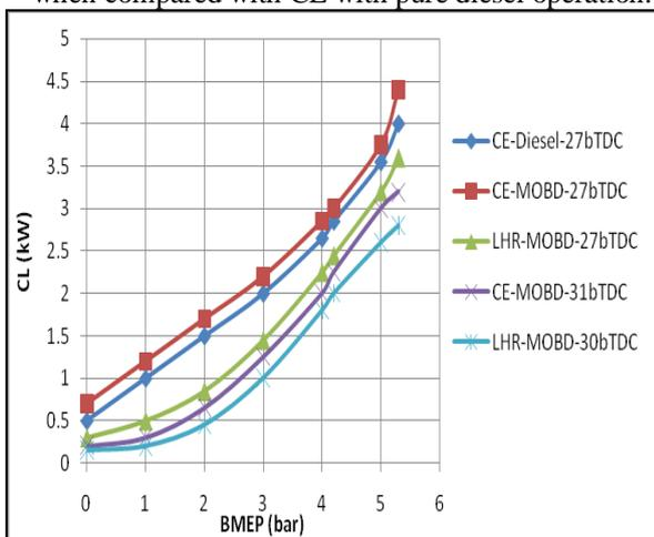
**Fig.10 Variation of coolant load (CL) with BMEP in both versions of the engine at recommended and optimized injection timings with MOBD operation at an injection pressure of 190 bar.**
