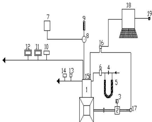
1.Engine, 2.Electical Dynamo meter, 3.Load Box, 4.Orifice meter, 5.U-tube water manometer, 6.Air box, 7.Fuel tank, 8, Pre-heater, 9.Burette, 10. Exhaust gas temperature indicator, 11.AVL Smoke meter, 12.Netel Chromatograph NO<sub>x</sub> Analyzer,
