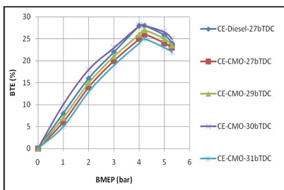
**Fig. 3. Variation of BTE with BMEP in CE at different injection timings with crude vegetable oil (CMO) operation**
