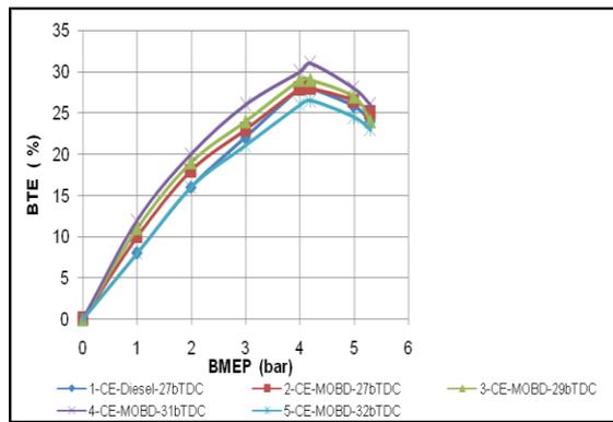
**Fig. 2 Variation of brake thermal efficiency (BTE) with brake mean effective pressure (BMEP) in conventional engine (CE) at different injection timings with mohr oil based bio diesel (MOBD) oil operation**
