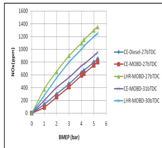
**Fig. 13 Variation of NOx levels with BMEP in CE and LHR engine at recommend injection timing and optimized injection timings with biodiesel (MOBD) operation.**
