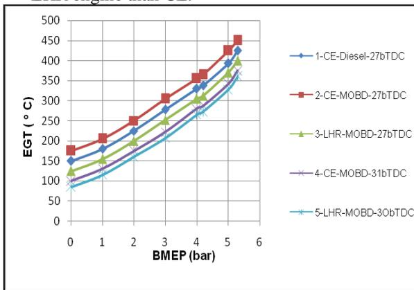
**Fig.8 Variation of exhaust gas temperature (EGT) with BMEP in CE and LHR engine at recommend injection timing and optimized injection timings with biodiesel (MOBD) operation.**
