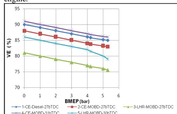
**Fig. 9 Variation of volumetric efficiency (VE) with BMEP in CE and LHR engine at recommend injection timing and optimized**
