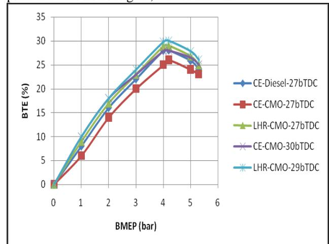
**Fig. 7 Variation of BTE with BMEP in different versions of the engine at the recommended injection timing and optimum injection timing at an injection pressure of 190 bar with CMO operation**
