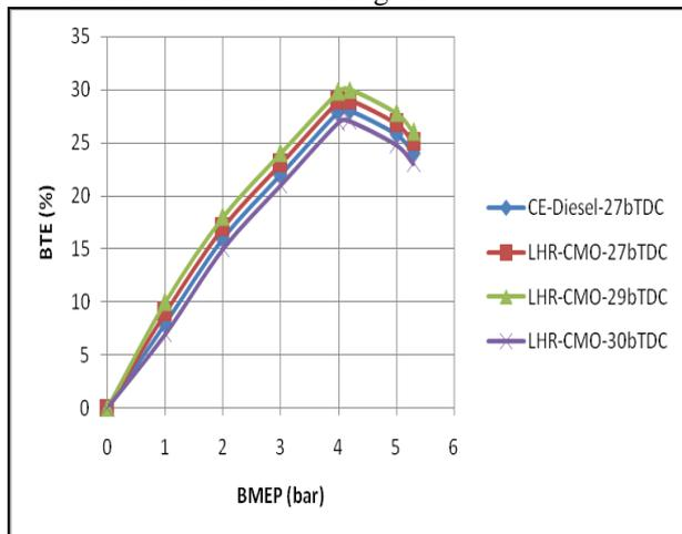
**Fig. 5 Variation of BTE with BMEP in LHR engine at different injection timings with crude vegetable oil (CMO) operation.**
