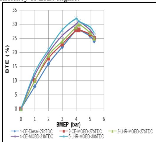
**Fig. 6 Variation of BTE with BMEP in different versions of the engine at the recommended injection timing and optimum injection timing at an injection pressure of 190 bar with biodiesel (MOBD) operation.**
