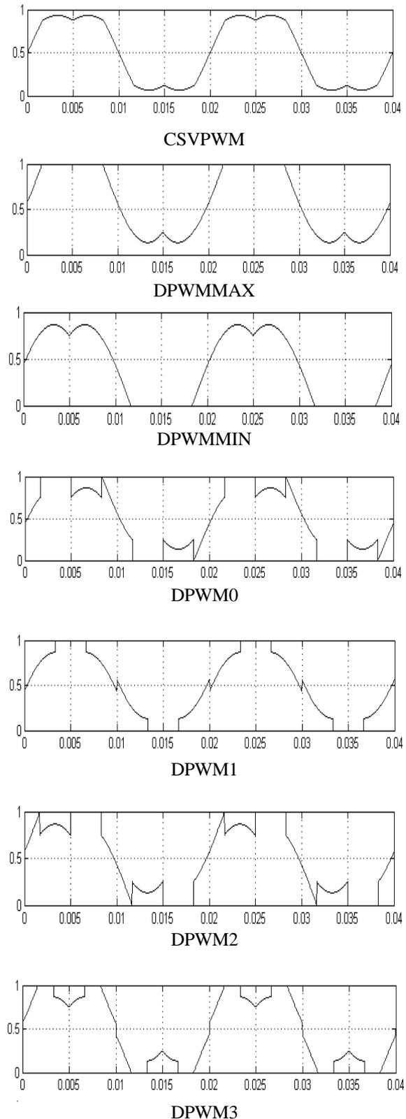
**Figure-1** Modulating waveforms of different sequences
