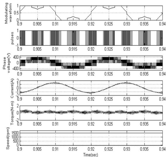
Figure 4.7 Steady state transients of DPWM3
