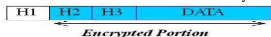
Fig. 11. Network Layer Encryption. In this case, data and more headers are encrypted. Here H1, H2 and H3 are headers.
