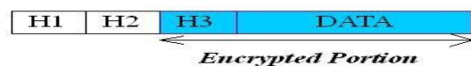
Fig. 12. Transport Layer Encryption. In this case, data and less headers are encrypted. Here H1, H2 and H3 are headers.
