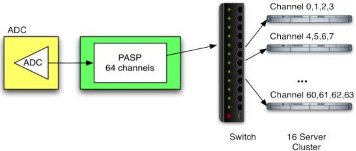
Figure 1: Example high level instrument architecture.
