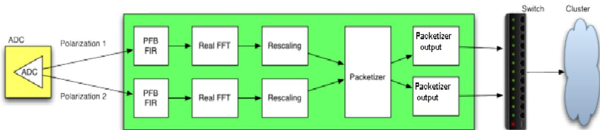
Figure 2: PASP Data flow design
