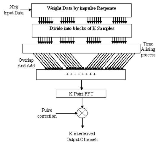
The implementation of WOLA DFT structures is as shown in the above figure where all lines represent complex data. The input sample is divided into frames of  $D$  samples and they are passed into a delay line. After they are weighted by the filter impulse response, then it is divided into blocks of  $K$  samples and overlapped to pass through the FFT. Finally the phase of the outputs is corrected.
