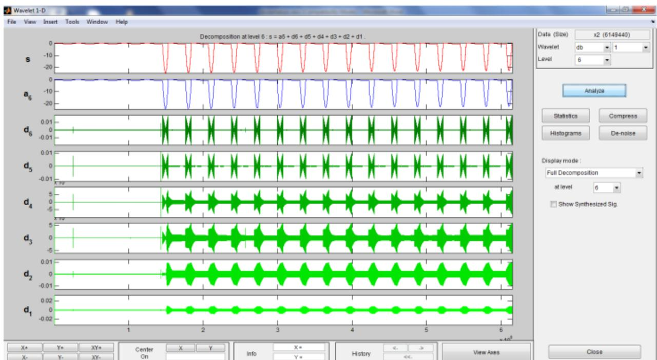
Fig.6 (b) WT of Diff. current for Magnetizing Inrush current at phase B.
