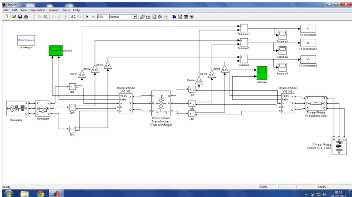
Fig.5 Implementation of Power system model under investigation in MATLAB
