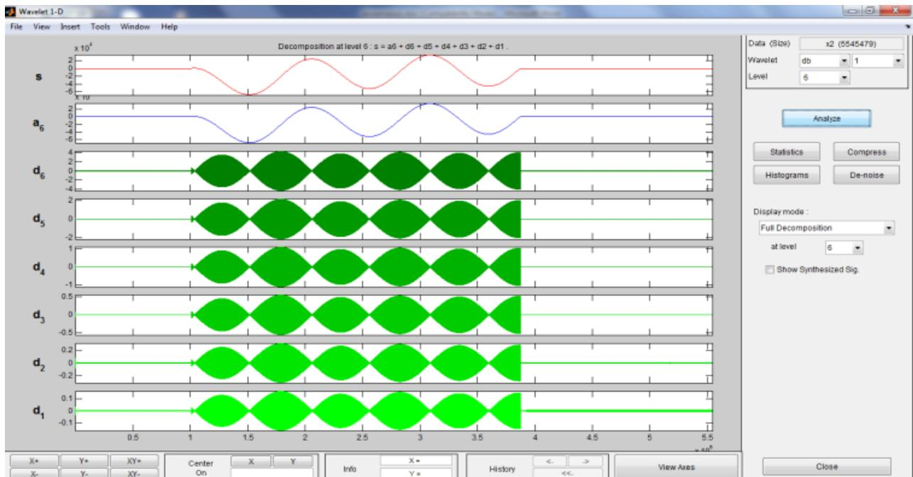
Fig.8. (b) WT of Diff. current for internal fault at phase B.
