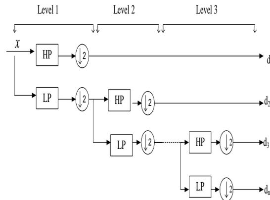
Fig.2. DWT multi-filter bank framework.
