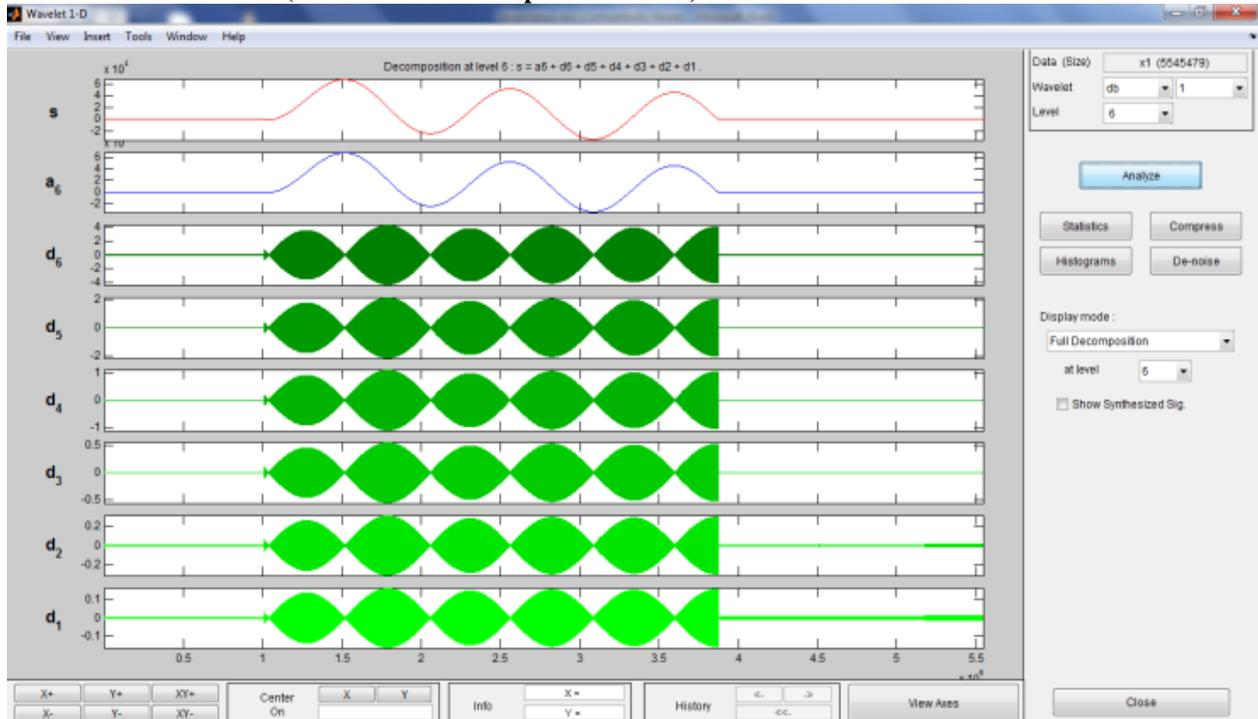
Fig.8. (a) WT of Differential current for internal fault at phase A.
