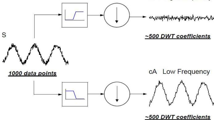
Fig. 1. Analyses of signal using wavelet transform
