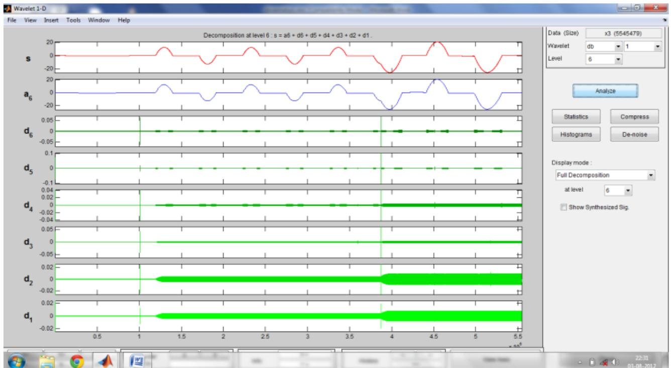
Fig.7 (b) WT of difference current for over excitation at faulty phase C.
