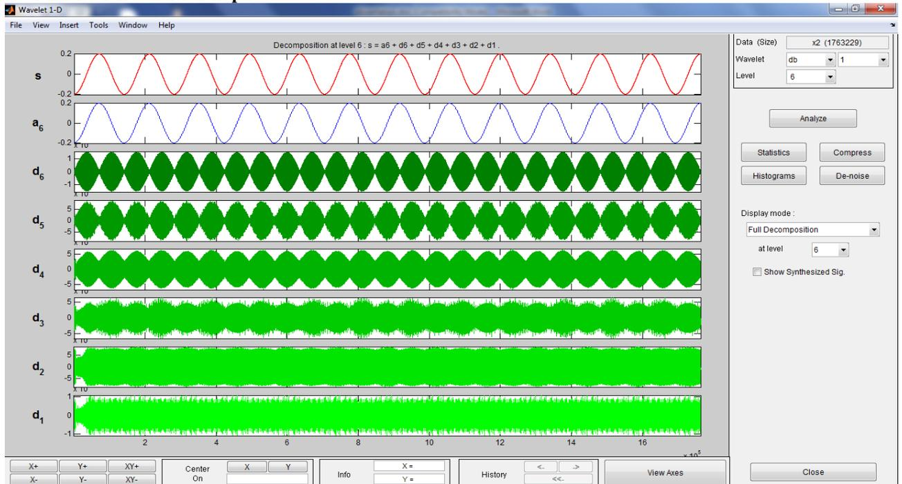
Fig.7 (a) WT of Differential current at healthy phase.
