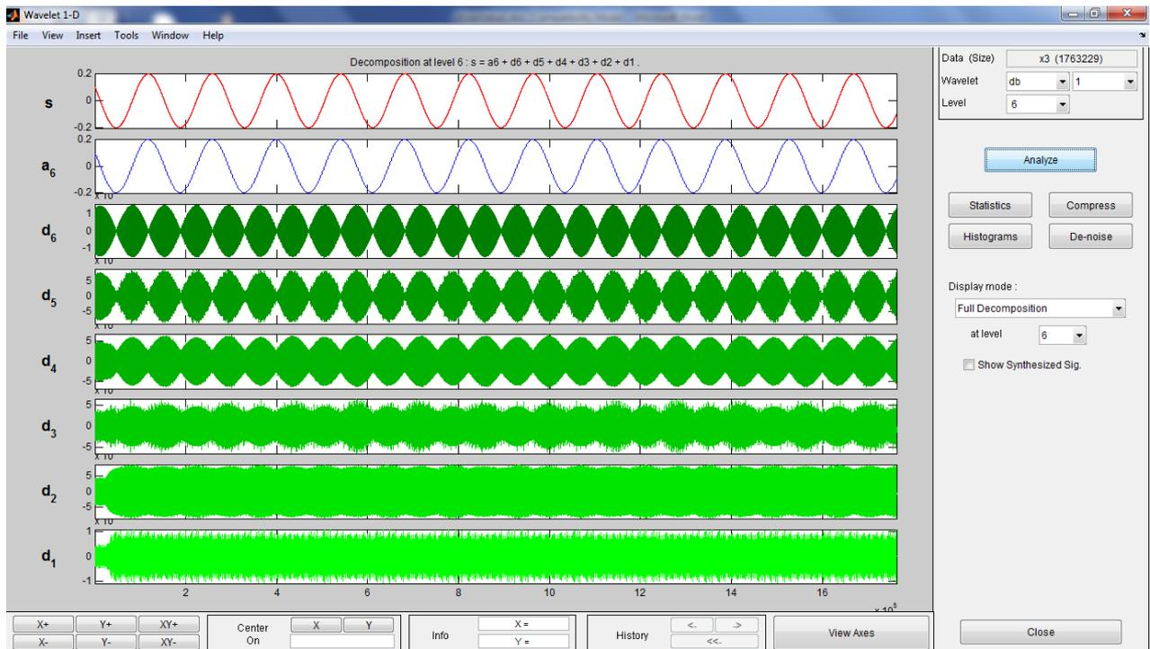
Fig.6 (c) WT of Difference current at phase C.
