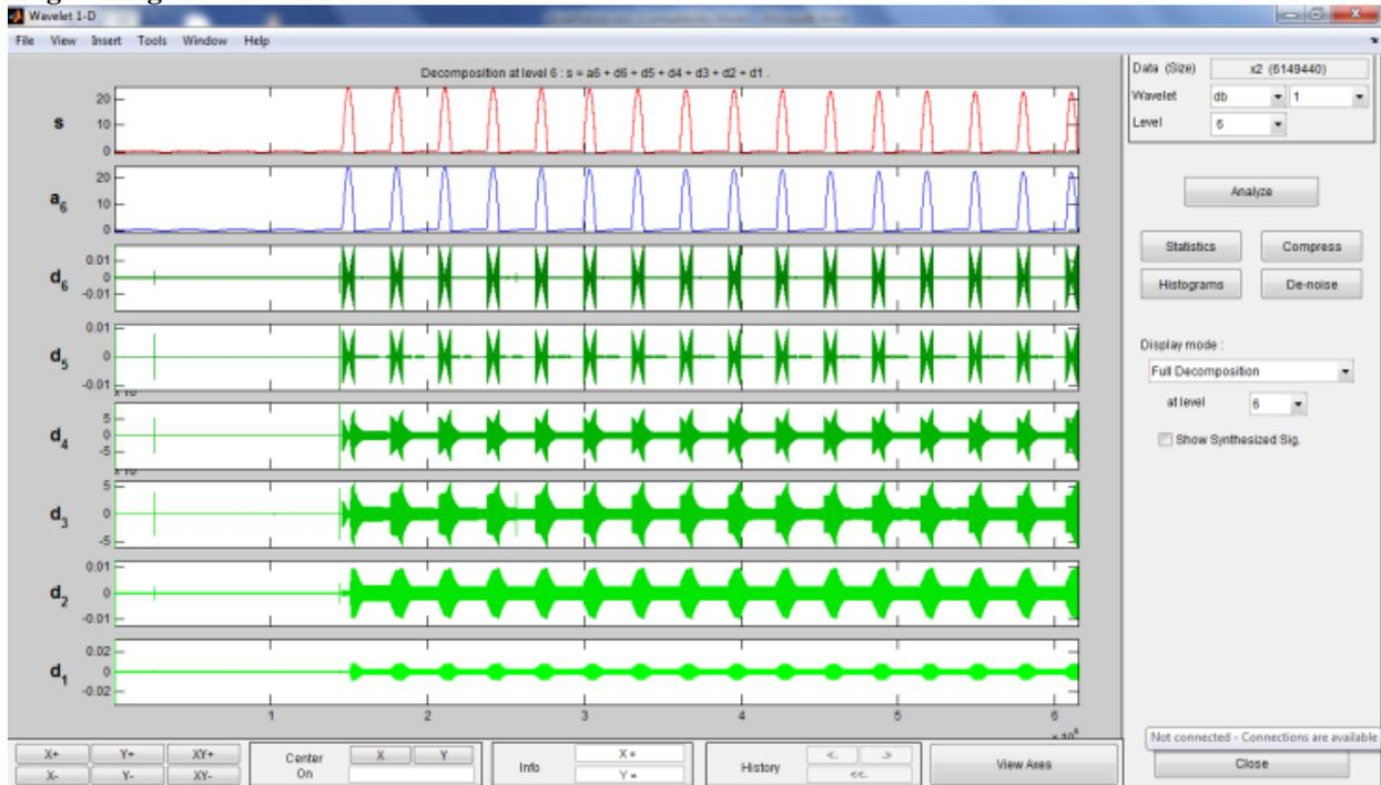
Fig.6 (a) WT of Diff. current for Magnetizing Inrush current at phase A.
