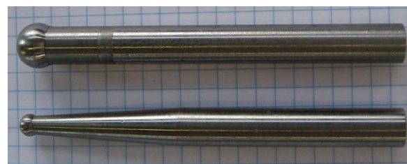
Fig.3. Forming tools for SPIF process [01]
