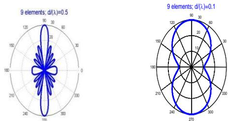
Fig.5: Radiation Pattern of conventional linear array
