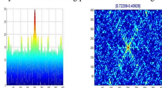
Fig 11: Array Factor plot and Radiated Field for sierpinski gasket
