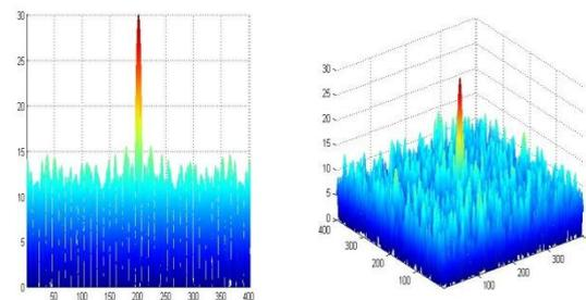
Fig.10: Array Factor plot for Random Array in 2D & 3D view
