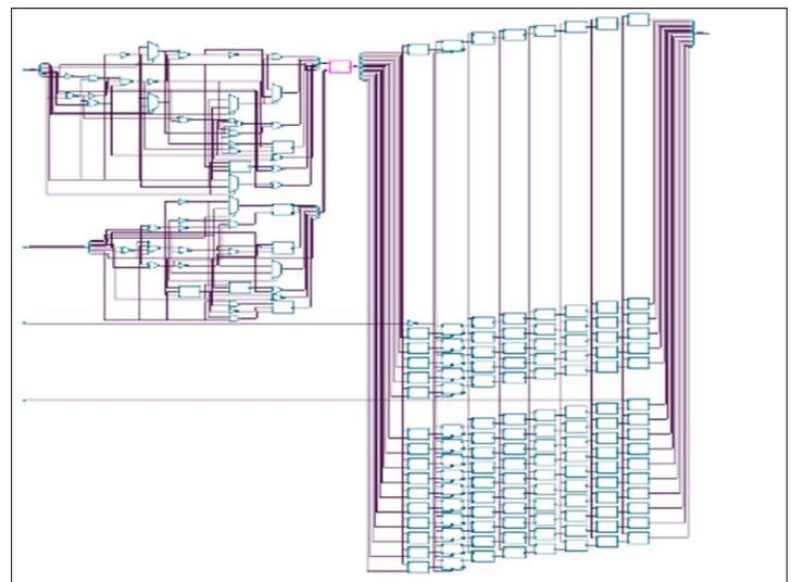
Fig.16 Pipelined Array Multiplier
