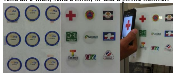
Fig. 4. RFID Stickers (Left). Emergency signs (Center). A user taps the red cross icon attached onto NFC RFID sticker tag, the sticker tag can be read if passed near a reader (Right).
