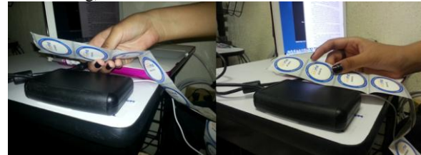
Fig. 3. Multi-ISO (OK 5553) RFID reader writing data on RFID stickers (Mifare DesfireTag)
