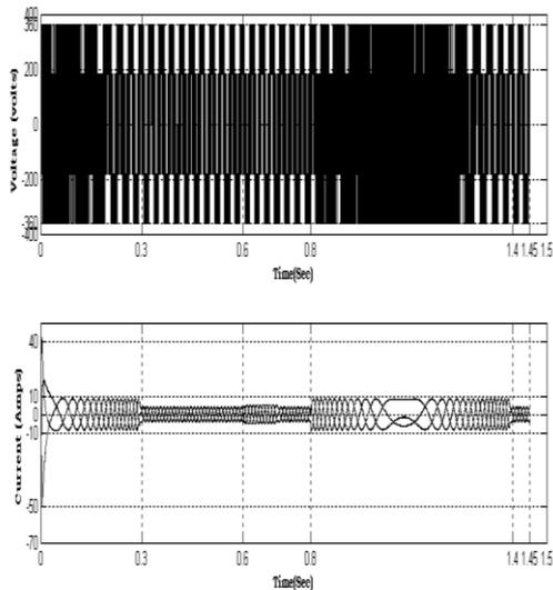
**Fig.14 Voltage and Current Plots for Proposed RPWM based DTC drive**
