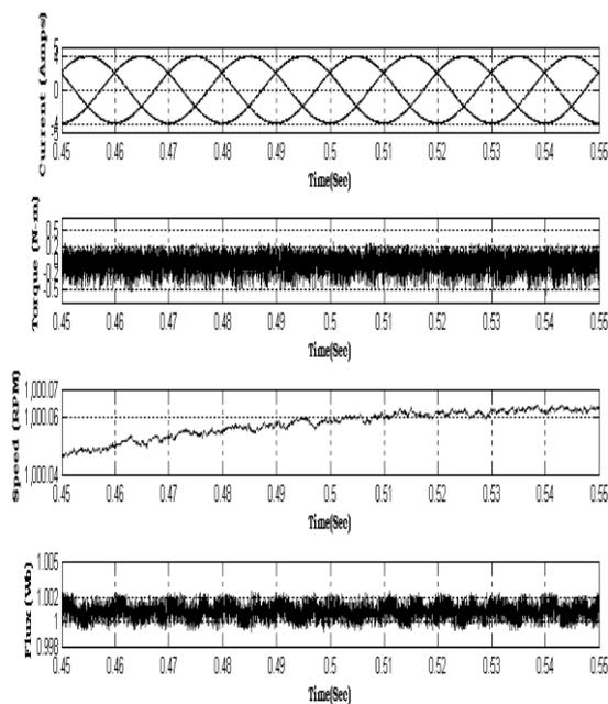
**Fig.11 Steady State Plots of Proposed RPWM based DTC drive**
