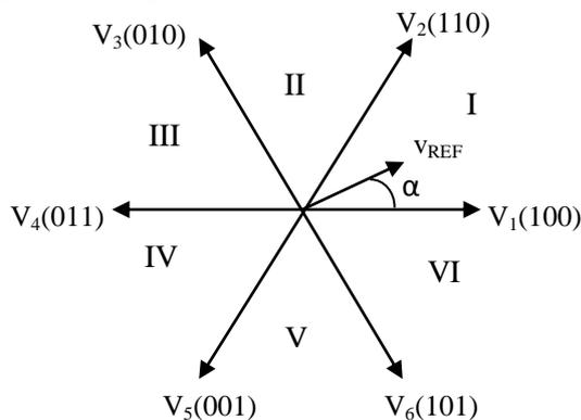
Fig.2 Inverter states o get and voltage vectors of three-phase inverter
