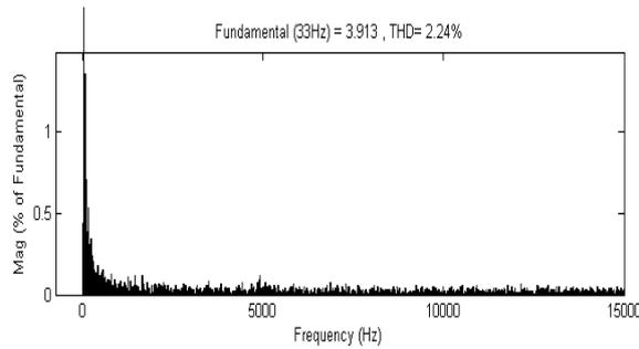
**Fig.9 Harmonic Spectra of line Current in Proposed RPWM based DTC drive**
