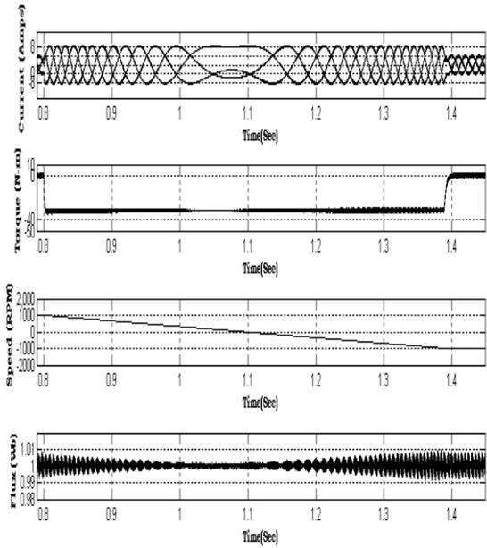
**Fig.6 Transients during speed reversal condition for SVPWM based DTC drive**
