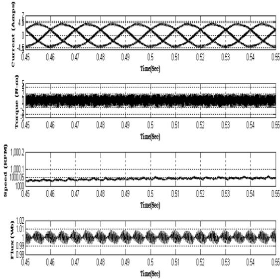
**Fig.4 Steady State Plots of SVPWM based DTC drive**
