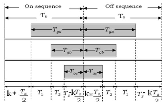
Fig-5. Gating signal generation using RPWM scheme in sector-I
