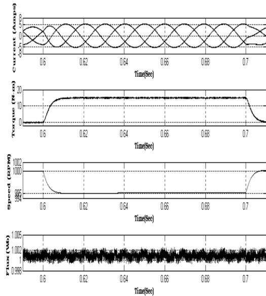
**Fig.12 Transients during step change in load for Proposed RPWM based DTC drive**
