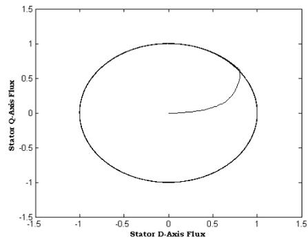
**Fig.8 Locus of Stator flux in proposed RPWM based DTC Drive**
