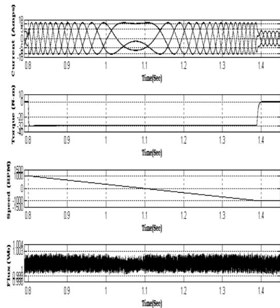
**Fig.13 Transients during speed reversal condition for Proposed RPWM based DTC drive**
