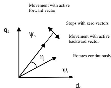
Fig.1  $\psi_s$  movement relative to  $\psi_r$  under influence of voltage vectors:
