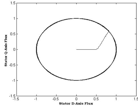
Fig.1 Locus of Stator flux in SVPWM based DTC Drive
