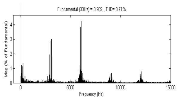
Fig.2 Harmonic Spectra of line Current in SVPWM based DTC drive
