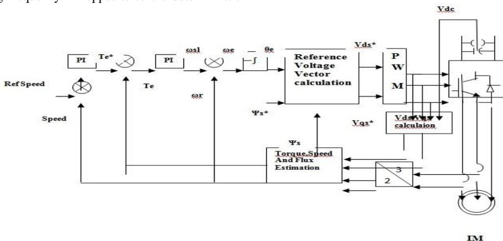
Fig-6 Block Diagram of RPWM based DTC
