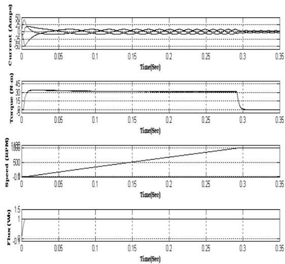
**Fig.10 Starting transients of Proposed RPWM based DTC drive**
