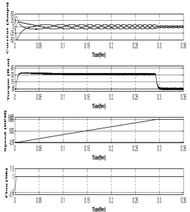
Fig.3 Starting transients of SVPWM based DTC drive
