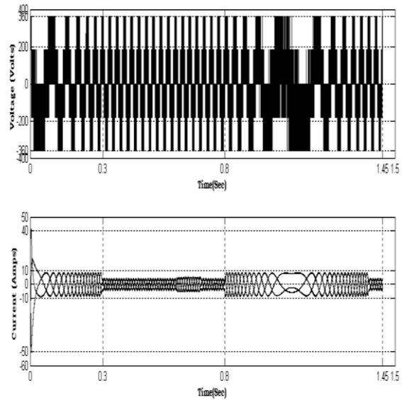
**Fig.7 Voltage and Current Plots for SVPWM based DTC drive**
