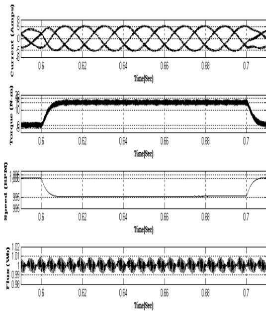
**Fig.5 Transients during step change in load for SVPWM based DTC drive**
