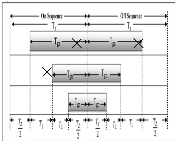
Fig-4. Gating signal generation using SVPWM scheme in sector-I
