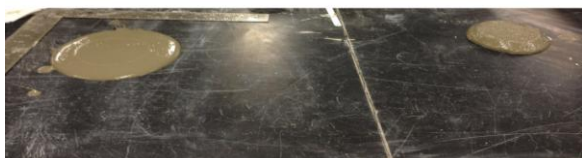
Figure 3: Flow ability test, control sample is on the left, and the sample with sodium polyacrylate is on the right.
