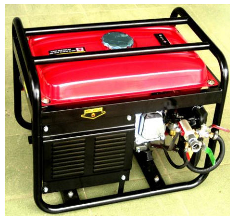
Figure 3. A forced ignition engine running on biogas was converted from a gasoline engine
