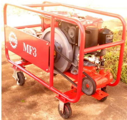
Figure 4. A dual fuel engine powered by diesel/ biogas -- converted from a diesel engine
