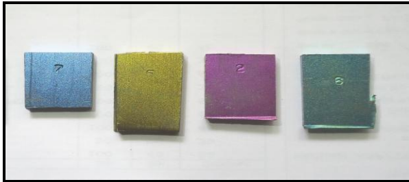
Fig 5: Titanium Spectrum at different voltage ranges in KOH bath
