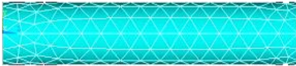
Fig. 3. A sample of a meshed Non-Prismatic beam with different small to large diameter ratio.
