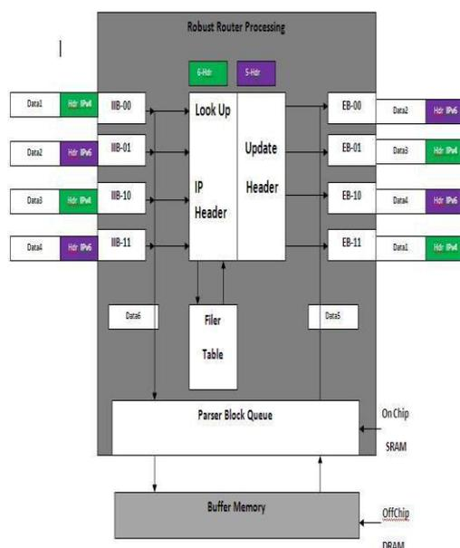
Figure 3 Multi-protocol Multi packet processing at a tree
