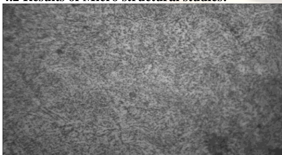
Fig. 2 : microstructure of base metal weld overlay with 160 welding speed
