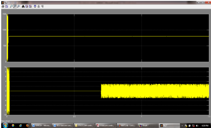
Fig. 7(a). The current through the dc link capacitor indicating the charging and discharging operation as shown in Fig. 7(b)
