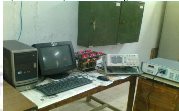
Fig.3: Experiment setup of 0.9 KVA, three phase transformer.
