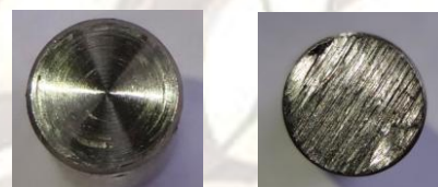
Fig.12. Fresh and Used Cylindrical Pin Surface
