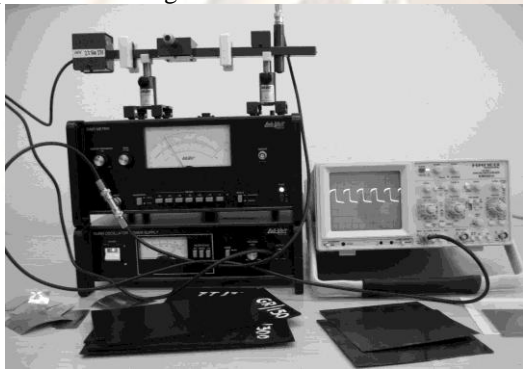
Fig. 3. The wave-guide-based measurement set-up for experimental determinations
