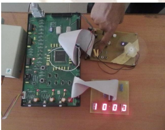
Fig. 6 Experimental setup of FPGA based PID controller for DC motor speed control.
